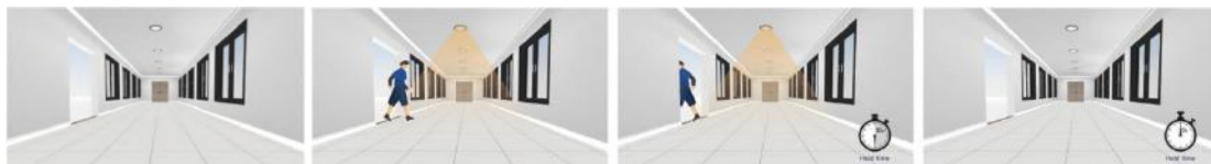
Turn off whole day if no motion Turn on whole day if motion Hold time count down Turn off after hold time
