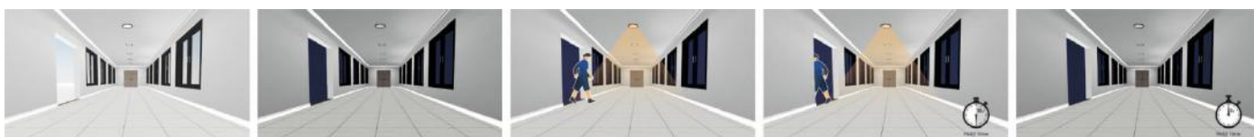
Turn off daytime Turn off night if on motion Turn on night if motion Hold time count down Turn off after hold time
