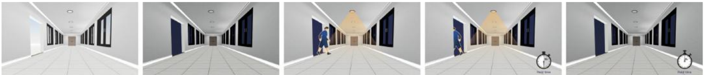
Turn off daytime Turn off night if on motion Turn on night if motion Hold time count down Turn off after hold time
