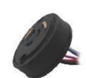
This series offers 2 gold-plated low voltage pads on the top surface to fit photocontrol has ANSI C136.41 conforming spring contacts, and offers 2 wiring leads at rear side for signal connection. Especially, this product does not occupy any space inside the lantern for those cases less internal space available.
